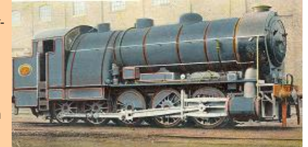
The experimental Great Eastern Railway Decapod—with 10 driving wheels it was the heaviest tank locomotive in Britain when built in 1902.
